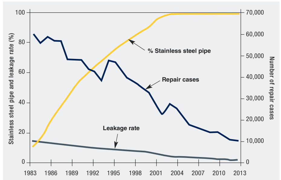
The relationship between stainless steel piping, leakage rates and repair cases in Tokyo's water system since 1983.
